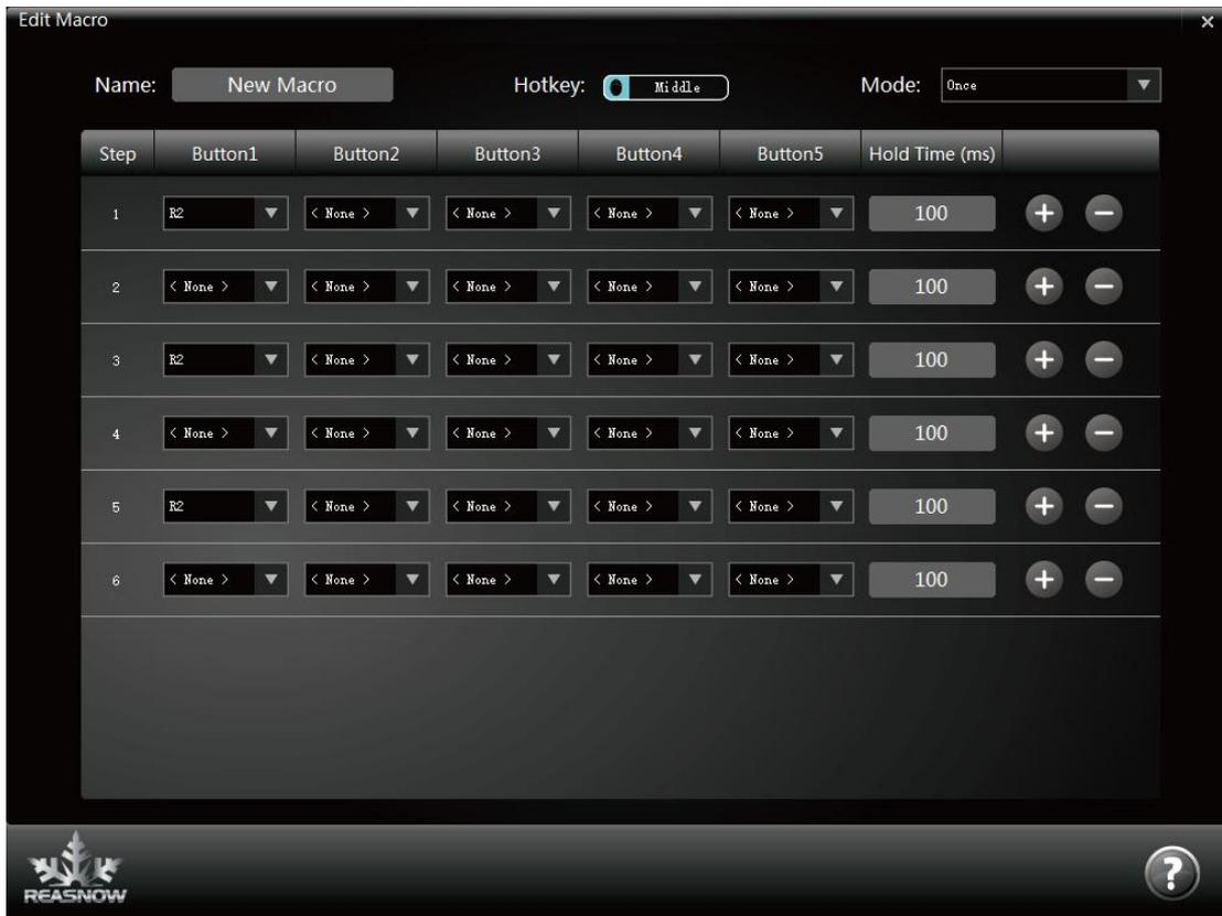
Here you can add 5 buttons, at the most, on controller to be activated at the same time, and set the corresponding Hold Time(ms) for these buttons.
